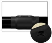
Weld in the welding plugs accordingly to the instruction of the plugwelder tool supplier. It is reccomended to heat up at the same time plug and the area around the hole for about 30 seconds at the heater temperature between  $220^{\circ}\text{C} - 230^{\circ}\text{C}$ . Perform the visual check of the finished joint connection
