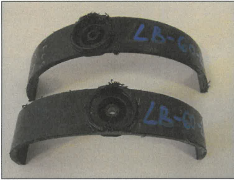
Photos 55, 56 Samples LB/60/2018 before bending test on welded plugs
