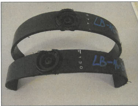
Photos 59, 60 Samples LB/16/2019 before bending test on welded plugs
